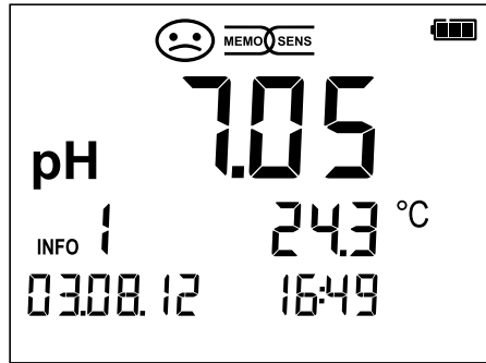
Example of a "Sensoface" message: INFO 1 (cal timer expired)
